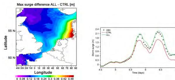
Figure 3: Left: Maximum surge difference in (m) during the storm Xaver between (a) coupled and NEMO model only; right: Observed (black squares) against computed storm surges for the circulation model only (red line) and the coupled wave-circulation model (green line) during storm Xaver at station Helgoland. The X-axis corresponds to the time in days from 01. December 2013
