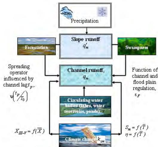
Figure 1. Block diagram of maximum runoff formation.
