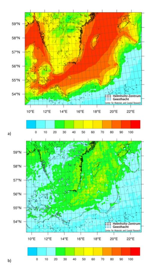
Figure 3: Change of  $NO_2$  concentrations (a) and N-deposition (b) in percent due to shipping (with — without ship emissions) for May 2012 in the Southern Baltic Sea region. It can be seen, that shipping according to the model is responsible for about 20 to 60 % of the  $NO_2$ -concentrations and up to 20-30% of nitrogen deposition in coastal land areas. Courtesy of Matthias Karl, HZG.
