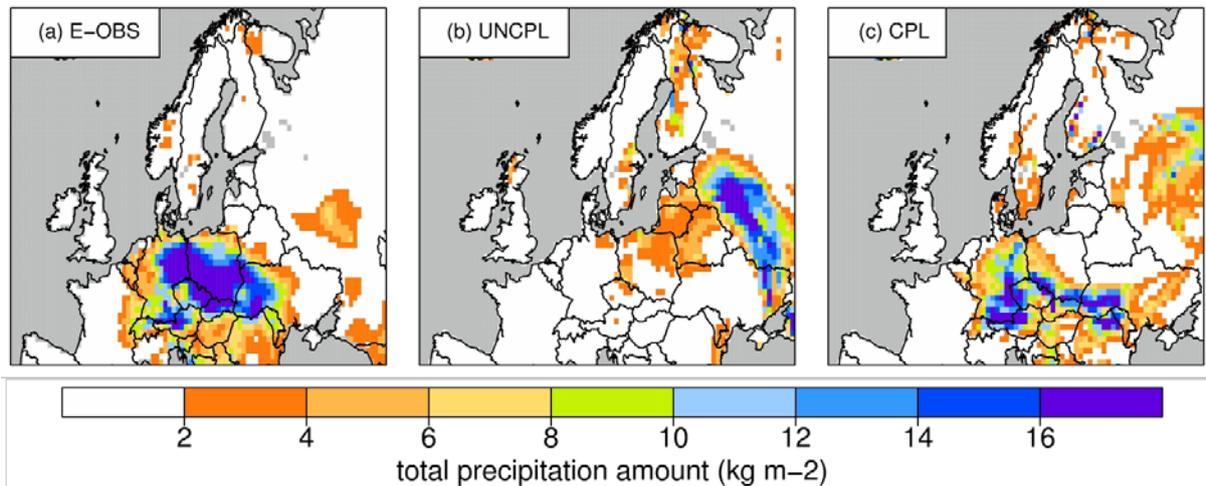
Figure: Mean precipitation (mm/day) of E-OBS data and simulated by the stand-alone atmospheric model COSMO-CLM and the coupled model COSTRICE averaged for 18-20 July 1997, the phase 2 of the Oder flood event. Taken from Ho-Hagemann et al. (2015).
