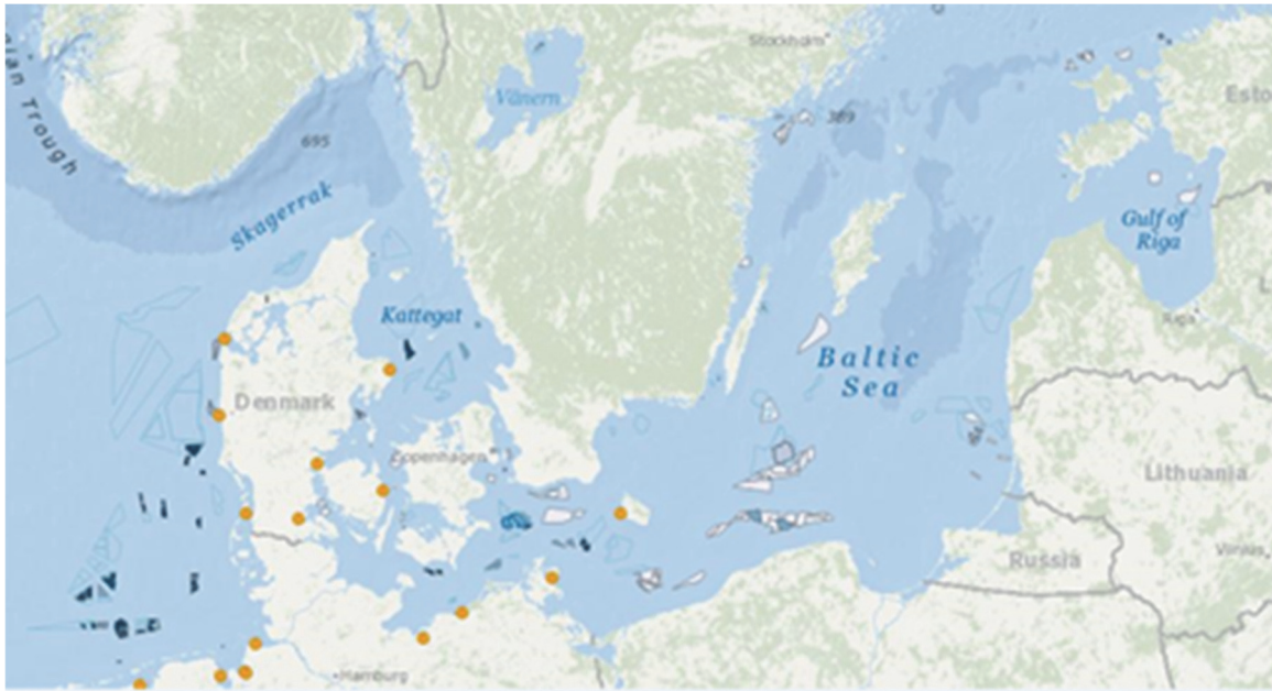
Fig. 13 Overview of wind farms over part of the Baltic and the North Sea, the dark blue are farms in operation, light blue are in construction and areas in blue lines are farms in planning (www.4coffshore.com).
