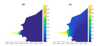
Figure 4. Dye distribution at the bottom layer of Oskarshamn harbor. The left one is taken at the first day and the right one is the  $300^{\text{th}}$  day.
