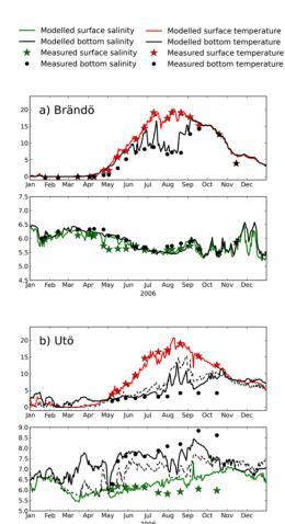
Figure 3. Modelled and measured temperature (upper panels) and salinity (lower panels) in two intensive monitoring stations a)Brändö (35 m) and b)Utö (68 m). Surface values are presented with colored lines and stars, bottom values with black lines and dots. For Utö, the dashed black line represents the bottom layer values from the simulation with older bathymetry grid.
