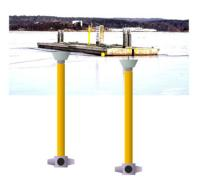
Figure 1. Pump used in the oxygenation experiment in the By Fjord. 2 m<sup>3</sup>s<sup>-1</sup> of surface water was pumped down to 35 m depth to oxygenate the deepwater, Stigebrandt et al. (2015a).
