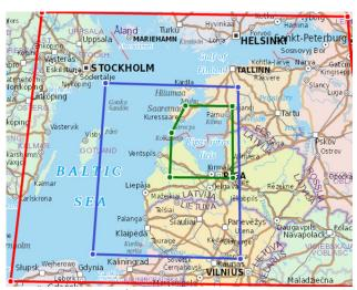
Figure 1. Setup area of HBM model. Red lines indicate area with rough mesh, blue lines finer mesh, green lines – assumed boundaries of Gulf of Riga
