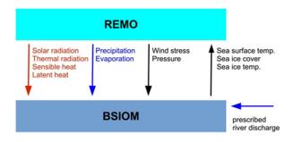
Figure 1. Coupling scheme of the model system
