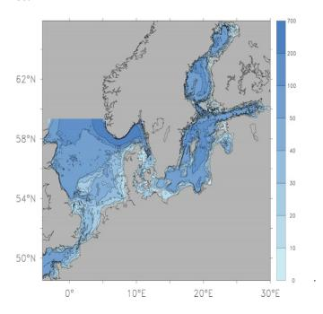
Figure 1. Bathymetry of the 2 nautical mile setup BASS02 of the shallow water model developed for this study.
